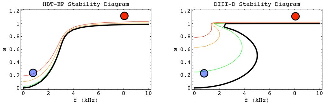
Figure 1: Open-loop stability diagrams characteristic of the HBT-EP and DIII-D tokamaks. The black curve represents marginal stability, and the orange and red curves represent exponential growth rates of 0.1, 0.5, and 1.0 msec<sup>-1</sup> respectively.
