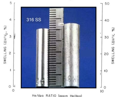
**Management of He transmutation products (matrix trapping at engineered 2nd phases) is a key factor for fusion materials**
