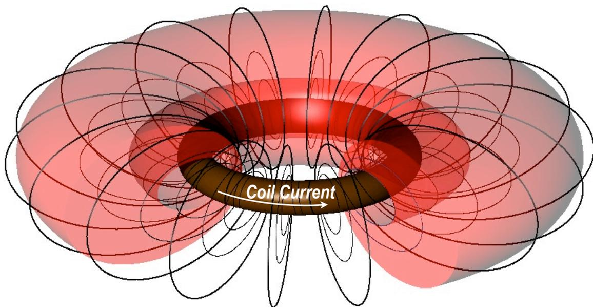
Poloidal Field from Toroidal Coil
