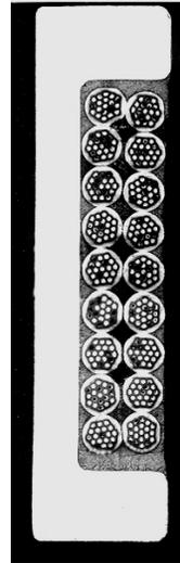
LDX Conductor in Soldered Cable
