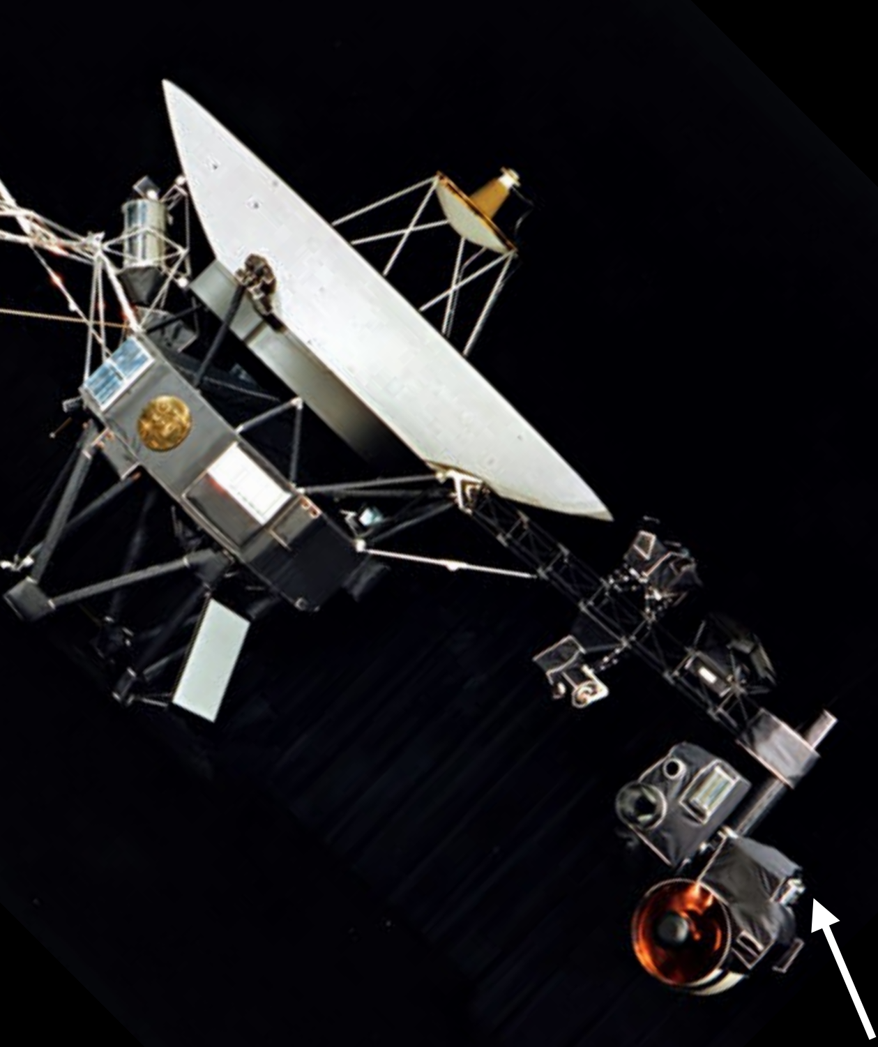
Plasma Science Experiment (PLS) Ions and Electrons: 10 eV – 5.9 keV
