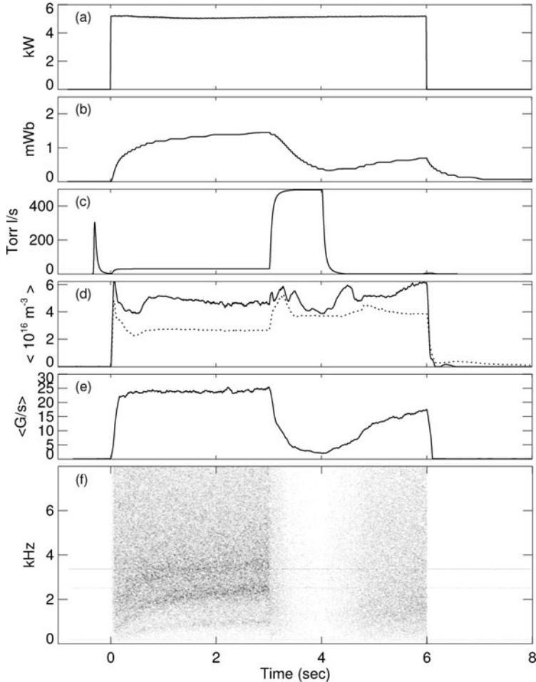
**Figure 4.** Traces for discharge 60714009 showing (a) ECRF heating power, (b) plasma diamagnetism, (c) neutral gas fueling rate, (d) two line-averaged densities from chords at  $R=0.77$  and  $0.96$  m (dotted), (e) ‘Mirnov’ magnetic fluctuation signal and (f) time–frequency-domain plot for this discharge.
