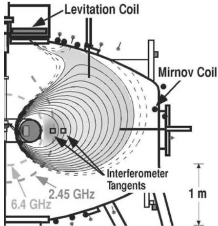
**Figure 1.** Schematic of the LDX experiment showing magnetic field lines, diagnostics and RF resonant surfaces at 2.45 and 6.4 GHz. An X-point ring null, or magnetic separatrix, is formed when the levitation coil is charged.
