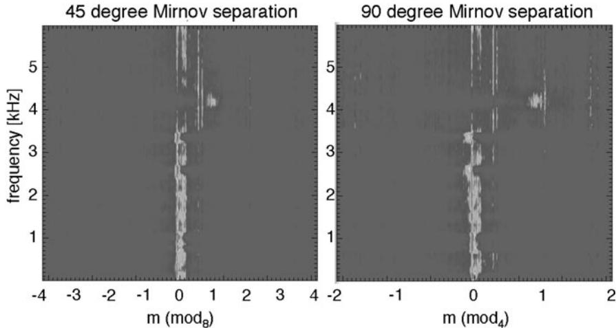
**Figure 3.** Correlation of Mirnov probes separated by  $45^\circ$  and  $90^\circ$  for discharge 60714020.
