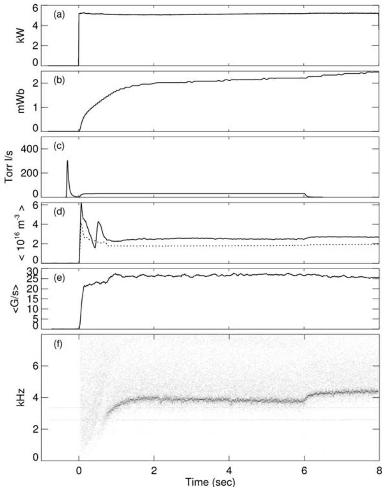
**Figure 2.** Traces for discharges 60714020 showing (a) ECRF heating power, (b) plasma diamagnetism, (c) neutral gas fueling rate, (d) two line-averaged densities from chords at  $R = 0.77$  and  $0.96$  m (dotted), (e) ‘Mirnov’ magnetic fluctuation signal and (f) time–frequency-domain plot for this discharge.
