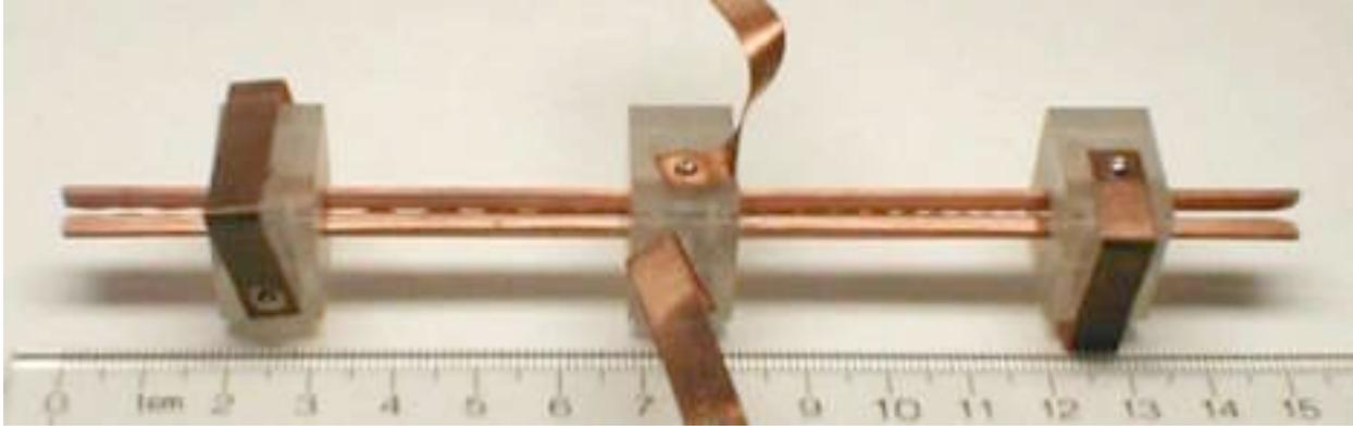
Fig. 5. 15 cm long RFQ accelerator used in experiments. Scallop wavelength increases by about 4.5 times from right to left, yielding a factor of 20 energy gain for accelerated ions.
