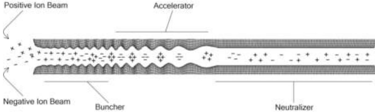
Fig. 1. Concept of production of energetic symmetric neutralized ion beam. Positive and negative ion beams are injected into an RFQ, where they are bunched and accelerated. The ions mix in the neutralizer, yielding a SNIB.
