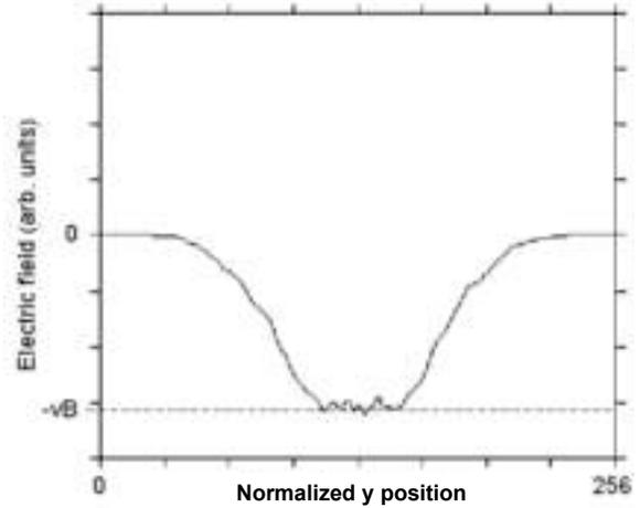
Fig. 4. Transverse electric field ( $E_y$ ) is plotted vs.  $y$  position within the beam. The electric field forms when the oppositely charged beam species separate in response to the magnetic field. Where the electric force negates the magnetic force ( $E_y = -vB$ ) the beam propagates undeflected.
