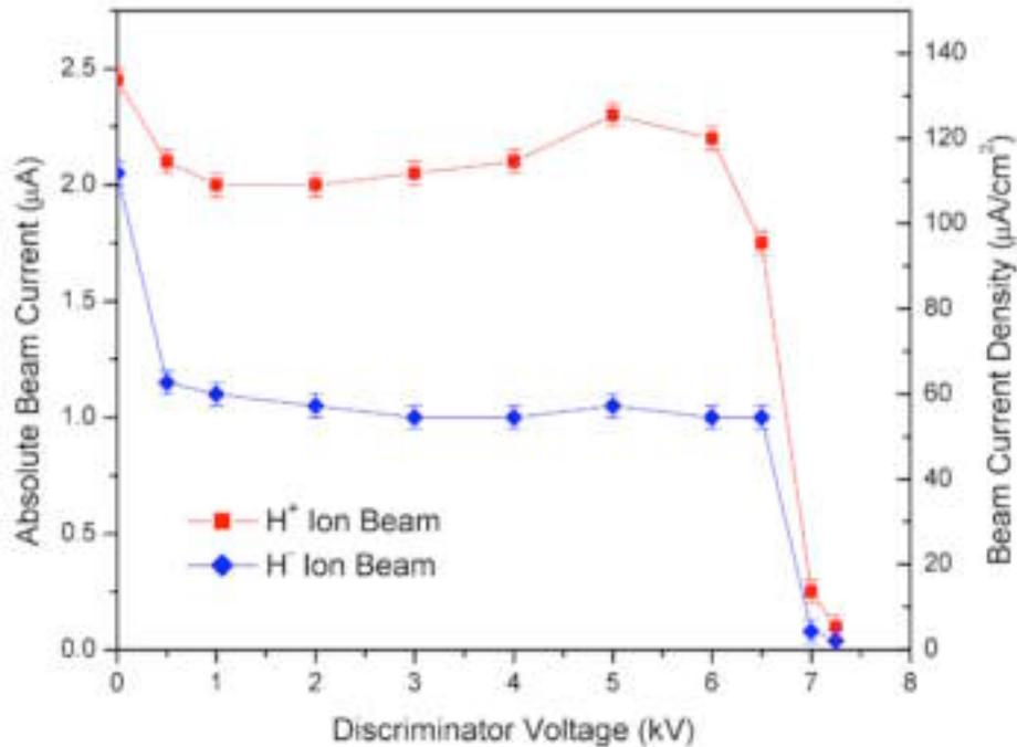
Fig. 6. Drop in current around 7 kV indicates H<sup>+</sup> and H<sup>-</sup> ion beams have about 7 keV energy, and have thus been successfully accelerated by the RFQ.
