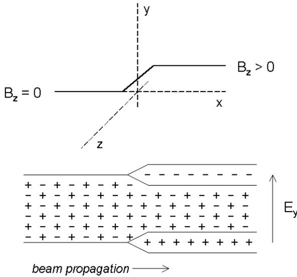
Fig. 3. Symmetric neutralized ion beam propagates across a transverse magnetic field. When the beam encounters the magnetic field, the positive and negative beam species are deflected in opposite directions. This forms charge layers, and the resulting electric field causes  $E \times B$  drift of the beam across the magnetic field.
