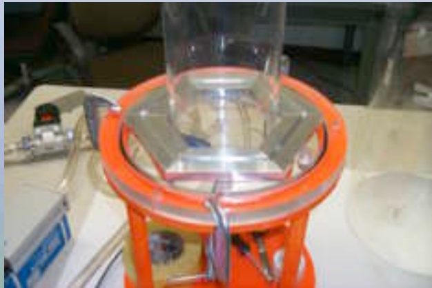
Grooved structure on the chamber floor
