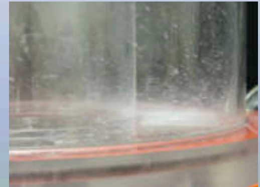
Wall deposits after mobilization
