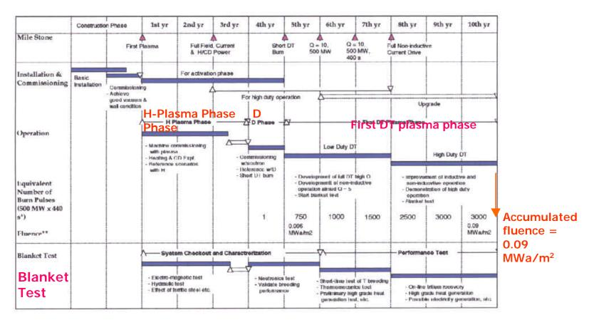
\* The burn time of 440 s includes 400 s flat top plus 40 s of full power neutron flux to allow for contributions during ramp-up and ramp-down \*\* Average fluence at first wall (neutron wall load is 0.56 MW/m<sup>2</sup> on average and 0.77 MW/m<sup>2</sup> at outboard equator)
