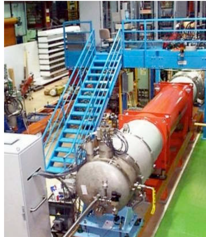
Test of Fermilab prototype quadrupole magnet for the LHC
