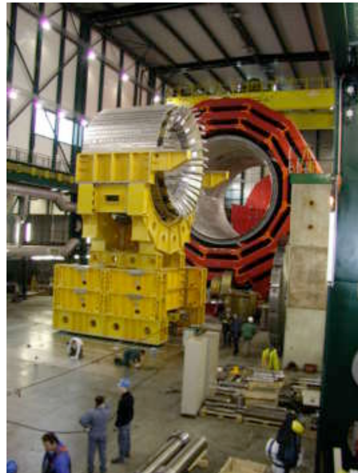
US-CMS-built hadron calorimeter module at CERN
