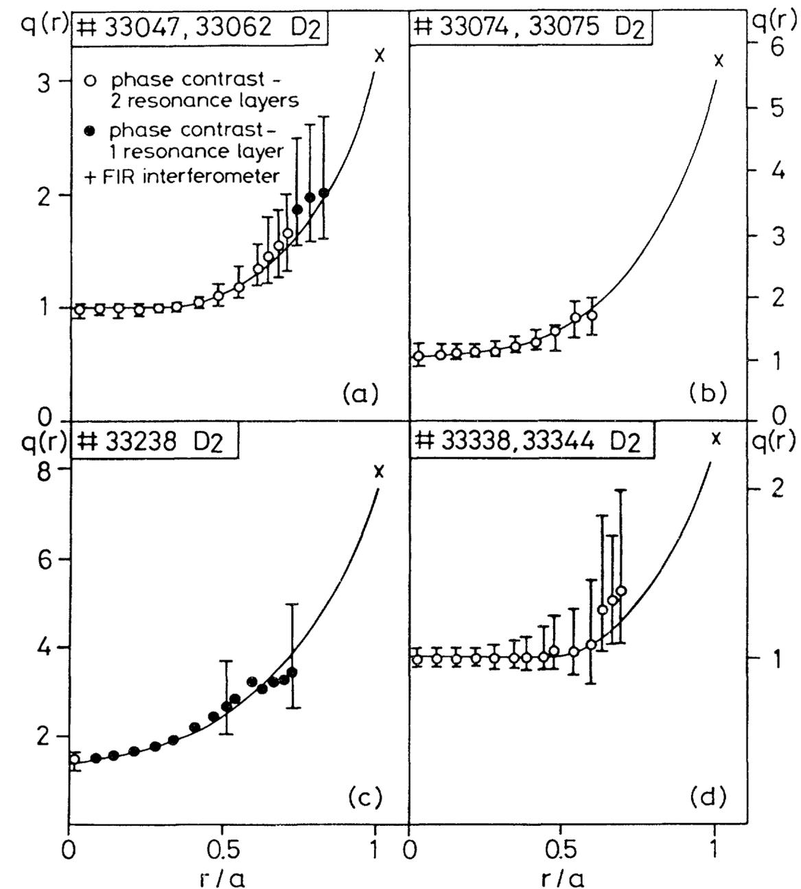
FIG. 5. Safety-factor profiles for (a)  $B_\phi = 1.51$  T,  $I_p = 125$  kA, (b)  $B_\phi = 1.51$  T,  $I_p = 70$  kA, (c)  $B_\phi = 1.51$  T,  $I_p = 50$  kA, (d)  $B_\phi = 1.16$  T,  $I_p = 135$  kA.
