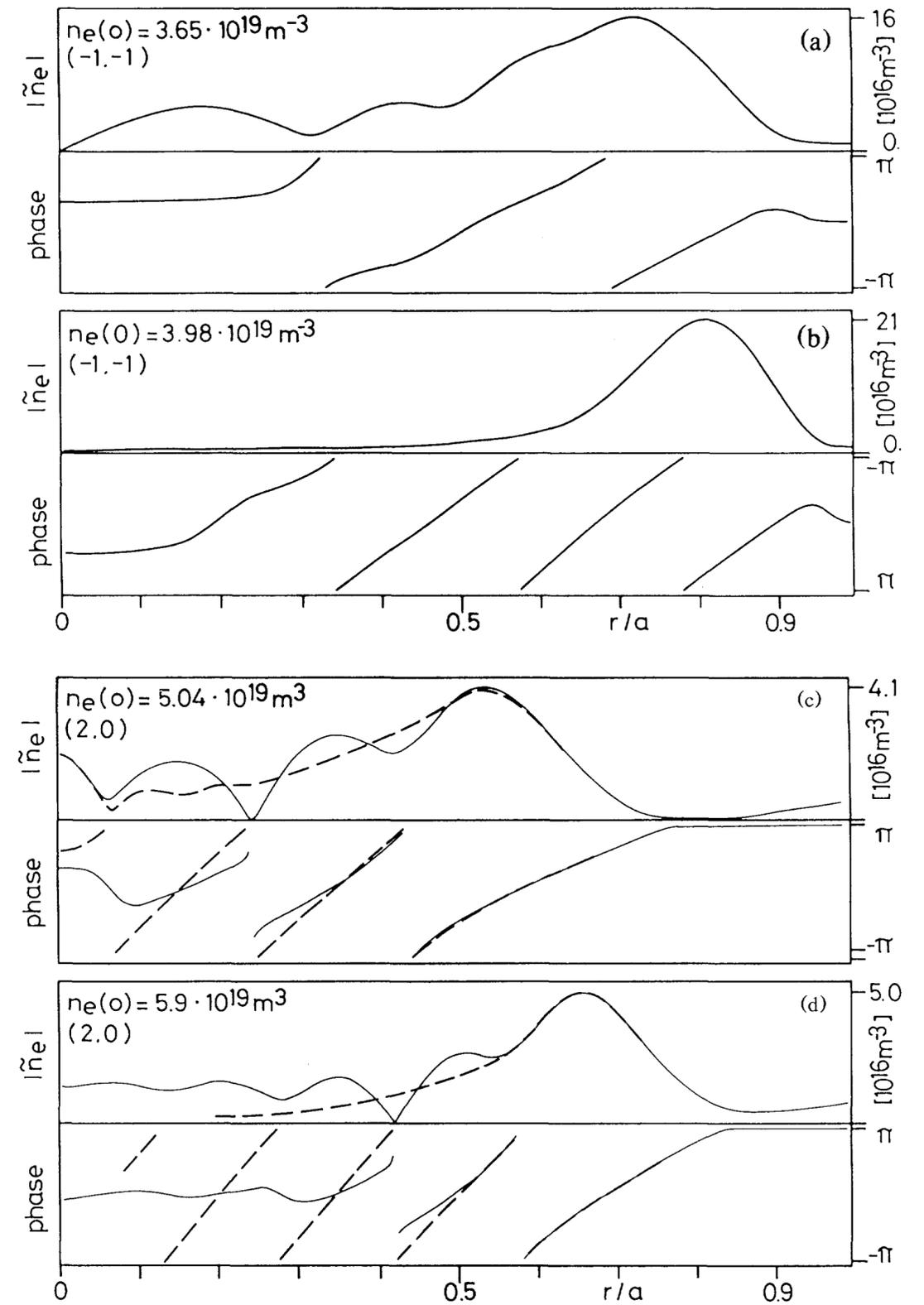
FIG. 3. Examples of calculated density fluctuations in the  $(-1, -1)$  and  $(2,0)$  continua. The resonance layer positions were chosen to match those of Fig. 2. The broken lines of (c) and (d) for the  $(2,0)$  KAW represent the remaining wave field after subtraction of the fast-wave mode.
