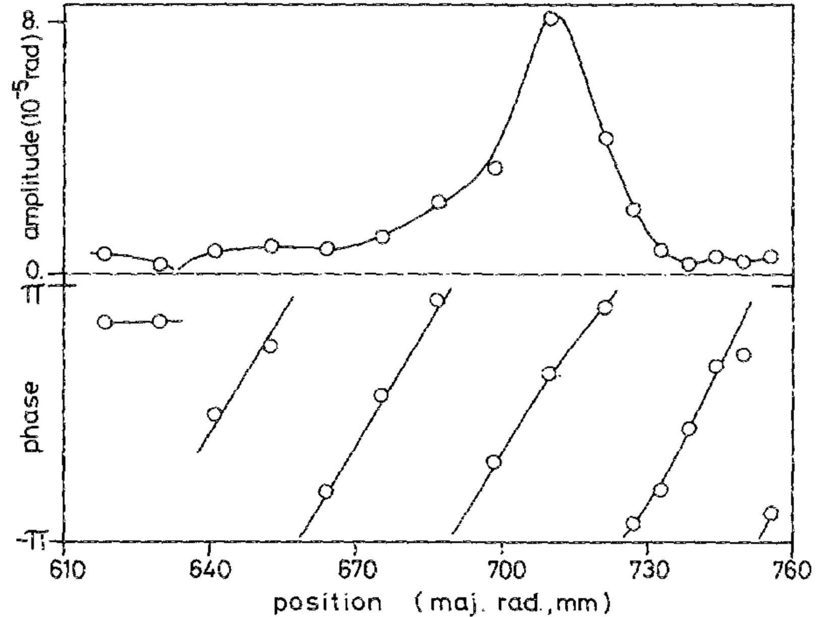
FIG. 10. Profile of amplitude and phase of synchronous density oscillations due to the kinetic Alfvén wave [(2, 0) continuum].
