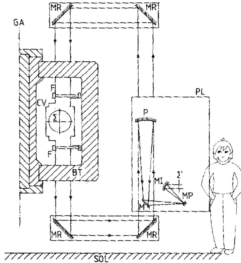
FIG. 3. Optical arrangement on the TCA tokamak. PL: optical table; P: parabolic mirror ( $f = 190.5$  cm); M: flat mirror; MP: phase mirror; MR: relay mirror; F: NaCl vacuum window; CV: vacuum chamber; BT: toroidal field coil; GA: major axis;  $\Sigma$ : object plane at plasma midplane;  $\Sigma'$ : image plane (imaging optics simplified).
