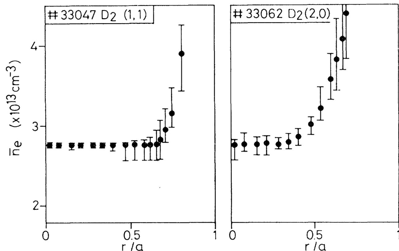
FIG. 4. Resonance layer positions for the (1,1) and (2,0) modes as a function of the central line density.
