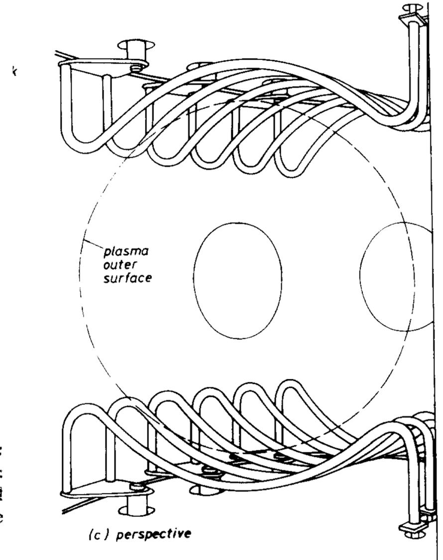
FIG. 1. Design of the TCA antennas: (a) vertical section, (b) horizontal section, and (c) perspective.
