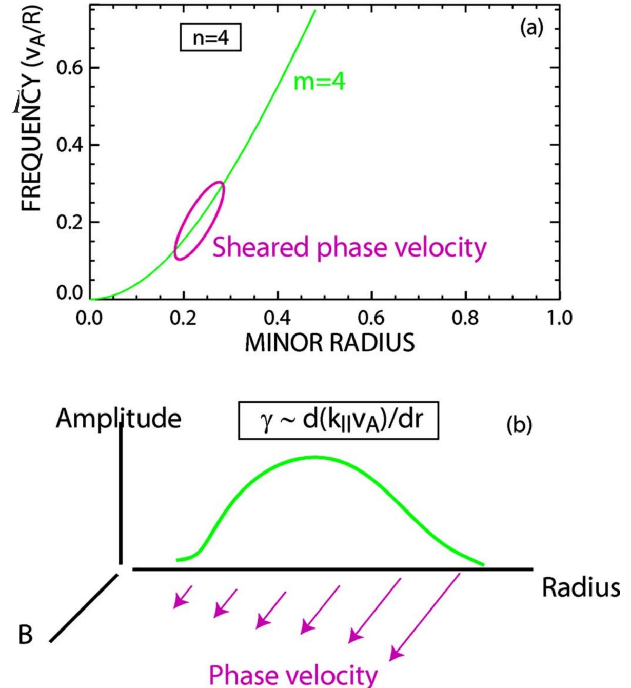
FIG. 1. (Color online) (a) Dispersion relation for an  $m=4$ ,  $n=4$  wave in a cylindrical plasma. The phase velocity is a strong function of radial position. (b) A hypothetical disturbance launched in the highlighted region. The pulse will rapidly disperse and shear.
