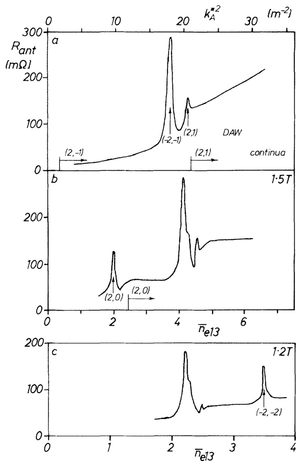
FIG. 1. Loading per antenna group as a function of line-averaged electron density ( $N=2$ ,  $M=1$ , deuterium plasma). (a) Cylindrical calculation; (b) measurements in standard conditions; (c) measurements at lower toroidal field and with side shields.
