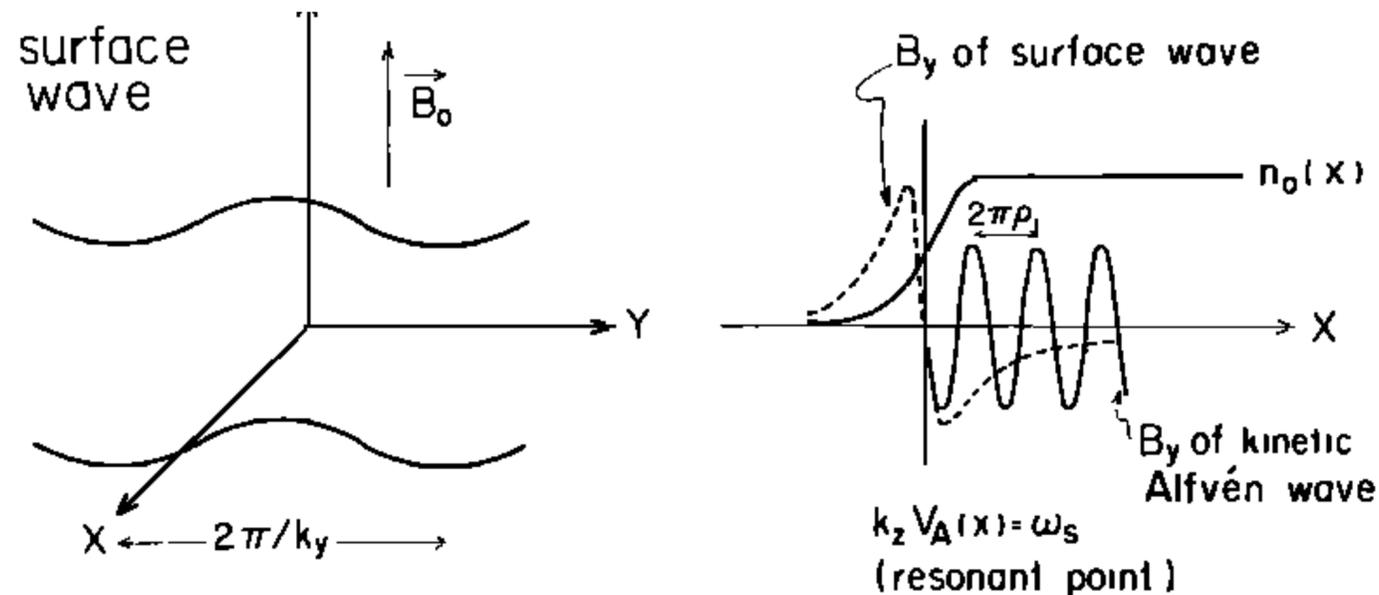
Fig. 1. Profile of the surface wave (left) and the amplitude variation of the surface and the kinetic Alfvén wave (right).
