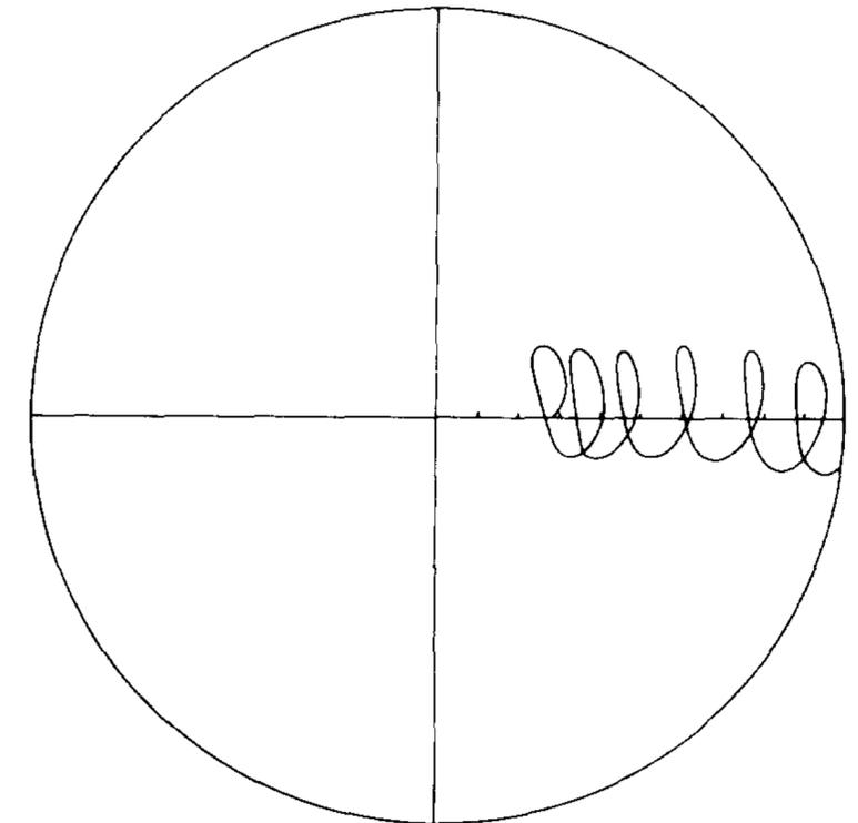
FIG. 5. A typical trajectory for a beam particle lost due to mode pumping. Here  $R_T = 35$  cm and the mode frequency is 20 kHz.
