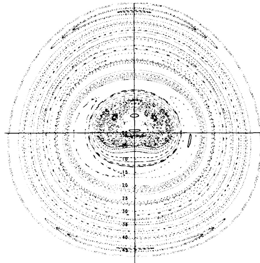
FIG. 3. The Poincaré plot of the magnetic field using the mode amplitudes approximating those given by the MHD simulation for a moderate fishbone. The  $n = 1$  modes are shown in Fig. 2. Also included were  $n = 2$  and  $n = 3$  modes, which at this amplitude have no appreciable effect on particle loss or energy. The figure extends to the plasma edge,  $r = 0.5a$ .
