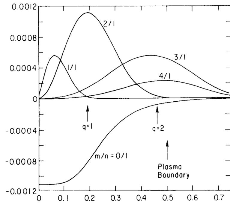
FIG. 2. Analytical approximations to the  $n = 1$  MHD modes for a moderate amplitude fishbone. The mode maximum and the value at the rational surface both agree with values given by the MHD simulation. Modes with  $n > 1$  were appreciably smaller.
