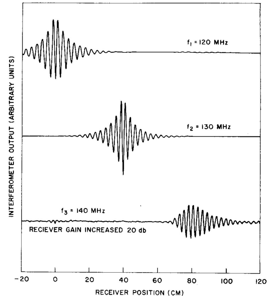
FIG. 2. Third-order echo. The transmitter probes are at 0 and 40 cm. Upper curve, receiver tuned to  $f_1$ ; second curve, receiver tuned to  $f_2$ ; third curve receiver tuned to  $f_3$  and gain increased 20 dB.
