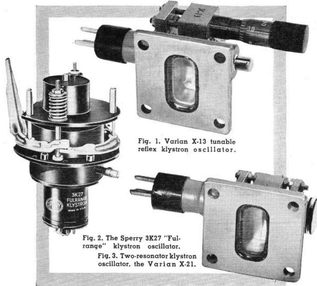
Fig. 1. Varian X-13 tunable reflex klystron oscillator.
