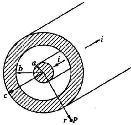
9. A coaxial cable having radii  $a$ ,  $b$ , and  $c$  carries equal and opposite currents of magnitude  $i$  on the inner and outer conductors. What is the magnitude of the magnetic induction at point  $P$  outside of the cable at a distance  $r$  from the axis?
