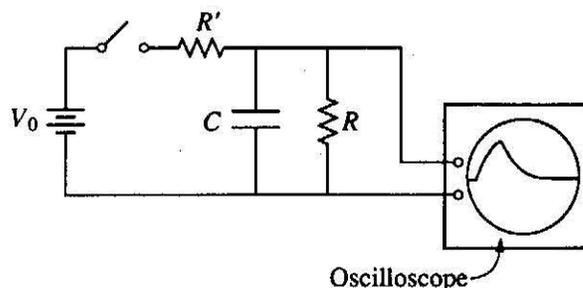
86. The circuit shown above is used to measure the size of the capacitance  $C$ . The  $y$ -coordinate of the spot on the oscilloscope screen is proportional to the potential difference across  $R$ , and the  $x$ -coordinate of the spot is swept at a constant speed  $s$ . The switch is closed and then opened. One can then calculate  $C$  from the shape and the size of the curve on the screen plus a knowledge of which of the following?
