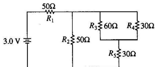
In the circuit shown above, the resistances are given in ohms and the battery is assumed ideal with emf equal to 3.0 volts.
