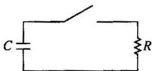
11. The capacitor in the circuit shown above is initially charged. After closing the switch, how much time elapses until one-half of the capacitor's initial stored energy is dissipated?
