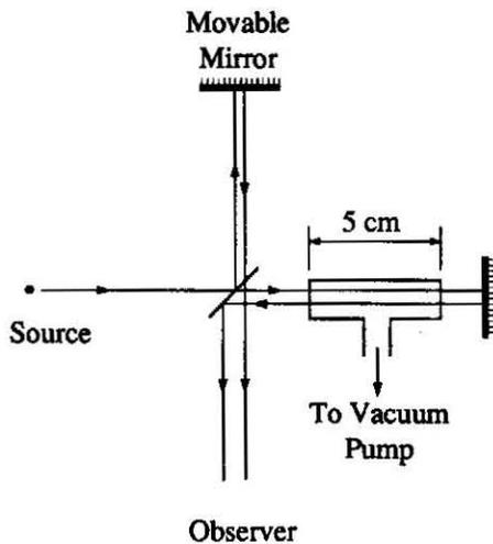
96. A gas-filled cell of length 5 centimeters is inserted in one arm of a Michelson interferometer, as shown in the figure above. The interferometer is illuminated by light of wavelength 500 nanometers. As the gas is evacuated from the cell, 40 fringes cross a point in the field of view. The refractive index of this gas is most nearly
