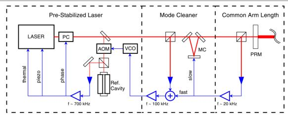
**Figure 4.** Schematic layout of the frequency stabilization servo. The laser is locked to a fixed-length reference cavity through an AOM. The AOM frequency is generated by a voltage controlled oscillator (VCO) driven by the MC servo, which is in turn driven by the common mode arm length signal from the REF port. The laser frequency is actuated by a combination of a pockels cell (PC), piezo-actuator and thermal control.
