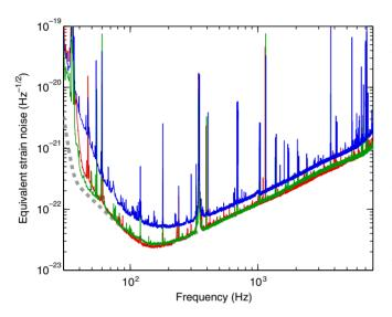
**Figure 6.** Strain sensitivities, expressed as amplitude spectral densities of detector noise converted to equivalent GW strain. The vertical axis denotes the rms strain noise in 1 Hz of bandwidth. Shown are typical high sensitivity spectra for each of the three interferometers (red: H1; blue: H2; green: L1), along with the design goal for the 4 km detectors (dashed gray).
