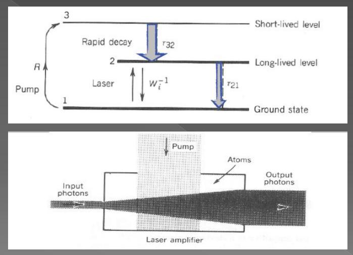
Example of a 3-level LASER system (still 2 level system where the actual Lasing happens.)
