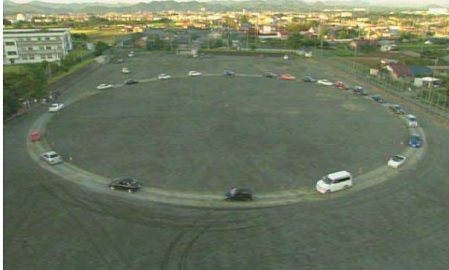
Figure 2. A snapshot of the experiment on a circular road. The circumference is 230 m, and the number of vehicles is 22. A 360-degree video camera is situated at the center of the circle for measurement.
