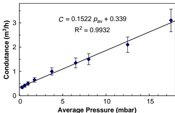
Fig. 4. Roughing line conductance as a function of average pressure at the ends of the line. The solid line represents a linear fitting to the data.
