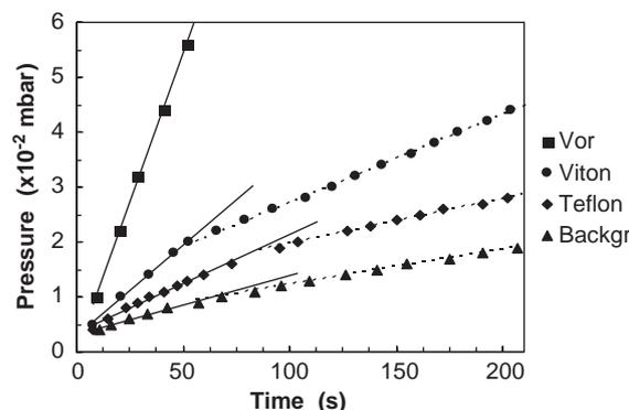
Fig. 5. Pressure rise in the high-vacuum chamber as a function of time, after the high-vacuum valve has been closed, for the different samples present inside the sample chamber. The solid and broken lines present linear fittings to the different data points in the lower and higher pressure regions, respectively.
