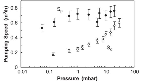
Fig. 3. Rotary pump pumping speed as a function of pressure at pump inlet ( $S_p$ ) and in the high-vacuum chamber ( $S_c$ ).
