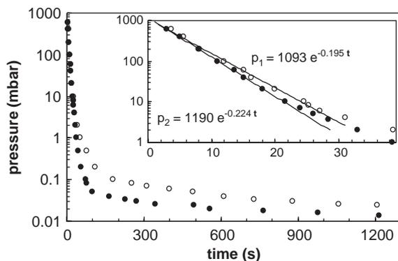
Fig. 1. Pressure evolution as a function of time in the high-vacuum chamber ( $p_1$ ) (○) and at the rotary pump inlet ( $p_2$ ) (●).
