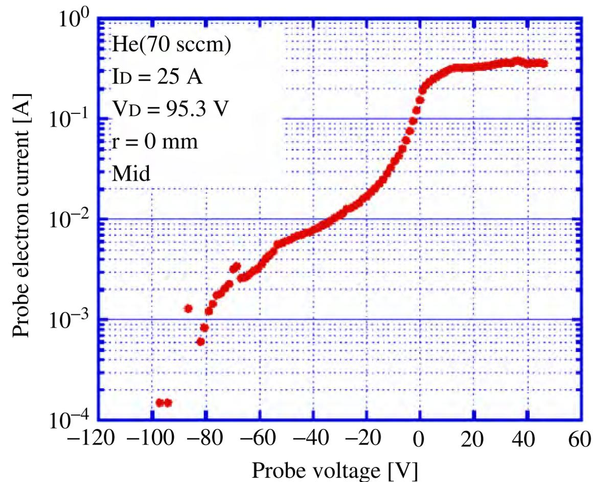
Fig. 11. Semilogarithmic plot of probe electron current versus probe voltage
