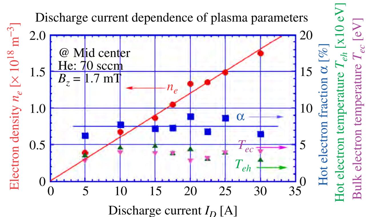
Fig. 12. Discharge current dependence of plasma parameters: the electron density, the fraction of hot electron component, and the temperature of bulk and hot electrons
