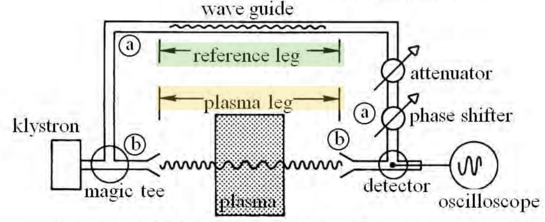
A microwave interferometer for plasma density measurement. 1.without plasma, signals from path and b are  $180^{\circ}$  out of phase. 2.with plasma, the phase in b changed as  $\lambda J$ , (by higher plasma density).
