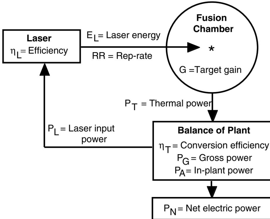
efficiency of  $\eta_T$ . Part of the gross electric power,  $P_G$ , is used for in-plant or auxiliary power,  $P_A$ , part is recirculated to operate the laser,  $P_L$ , and the remainder is the net power available for sale,  $P_N$ . The laser power is given by  $P_L = (E_L \times RR) / \eta_L$ , where  $E_L$  is the energy of all the laser beams, the  $RR$  is the laser repetition rate, and  $\eta_L$  is the laser efficiency.
