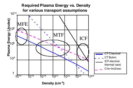
Figure 1. Required thermal energy in a plasma to achieve Lawson ( $n\tau \sim 3 \times 10^{14} \text{ sec/cm}^3$ ) as a function of density at T=10 keV, assuming a sphere for unmagnetized plasma, and an FRC geometry with plasma  $\beta = 1$  for magnetized plasma.
