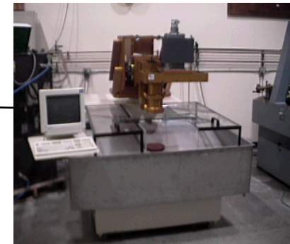
Lapping & Polishing (sub-surface damage, figure to 1µm Roughness to <50nm RMS)
