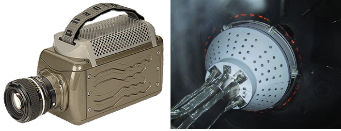
Figure 2.11: The Phantom v7.1 high speed digital video camera and the view-port through which the high-speed movies are taken (digital still photograph).
