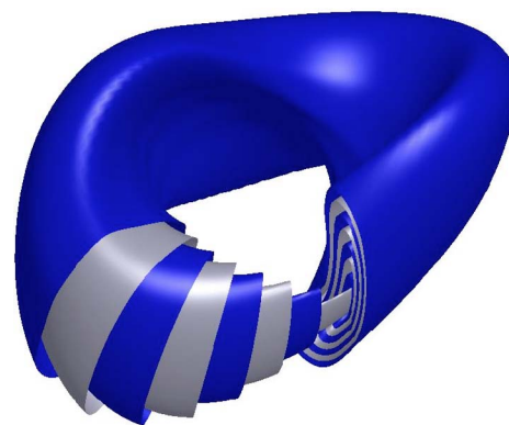
FIG. 7. (Color online). Cutaway view of the CNT magnetic surface configuration.
