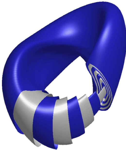
FIG. 1. (Color online) Cutaway view of the CNT magnetic surface configuration.
