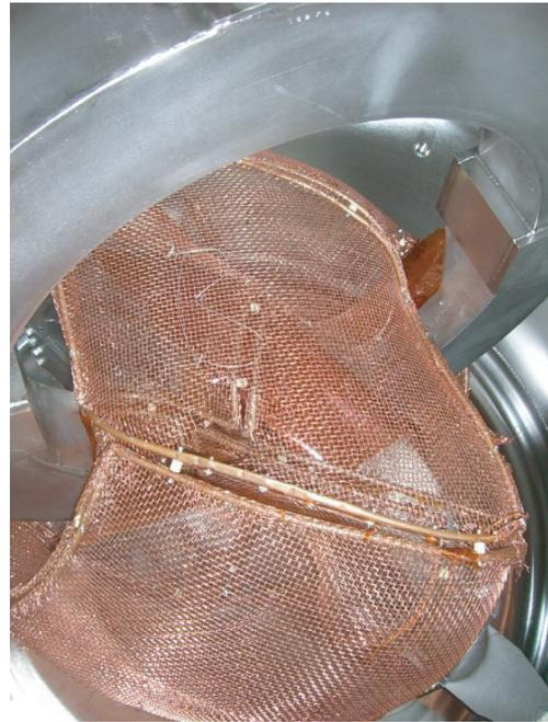
Fig. 3 The copper mesh electrostatic boundary installed in the CNT experiment.
