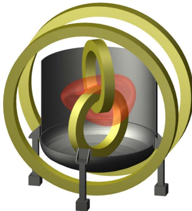
FIG. 3. (Color online) CAD drawing of the CNT device showing the complex boundary conditions set by the grounded vacuum chamber and coils.
