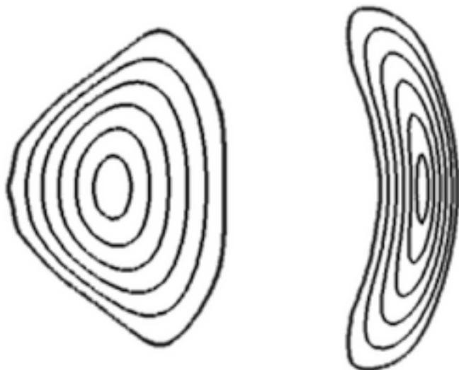
FIG. 2. Numerically calculated magnetic surface contours of the thick cross section at  $\phi=90^\circ$  (left) and the thin cross section at  $\phi=0^\circ$  (right). Compare to Fig. 1.
