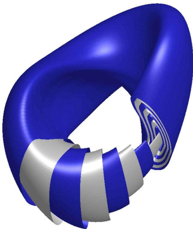
FIG. 1. (Color online) Cutaway view of the CNT magnetic surface configuration. The average major radius of the plasma is  $\approx 30$  cm and the average minor radius is  $\approx 15$  cm.
