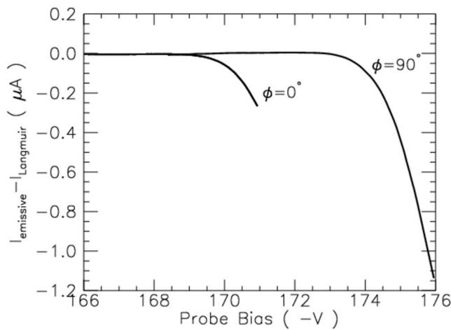
FIG. 4. The difference between the emissive and Langmuir probe characteristics is plotted as a function of the probe bias for probes at the  $\phi=0^\circ$  and  $90^\circ$  cross sections. The points where  $I_{\text{emissive}} - I_{\text{Langmuir}}$  becomes negative are the plasma potentials. There is clearly a potential difference between the two locations. For comparison with Table I, this is the 170 V emitter bias and temperature is  $T_e = 3.6 \pm 0.6$  eV.
