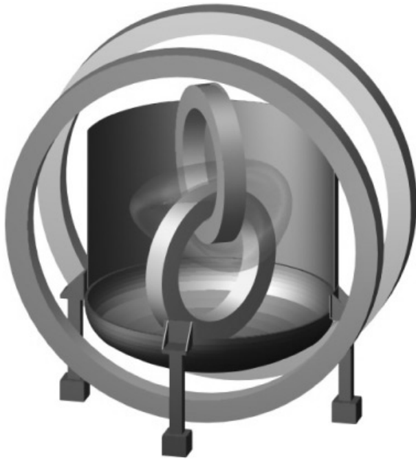
Fig. 1. The basic CNT configuration, showing the four coils and the resulting magnetic surface shaped inside the vacuum chamber.
