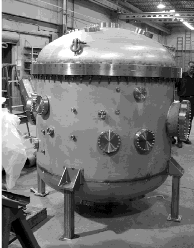
Fig. 7. The CNT vacuum chamber complete after leak tests at Ability Engineering in South Holland, Illinois.
