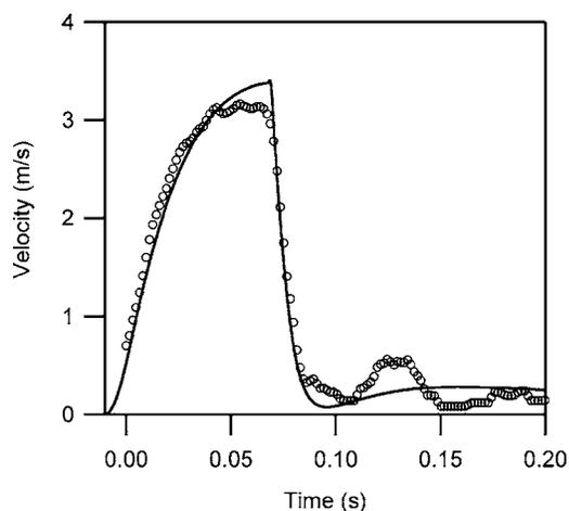
FIG. 7. Velocity vs time measurement and model for helium gas at 40 psig. The markers are the measured points and the line is the modeled velocity.
