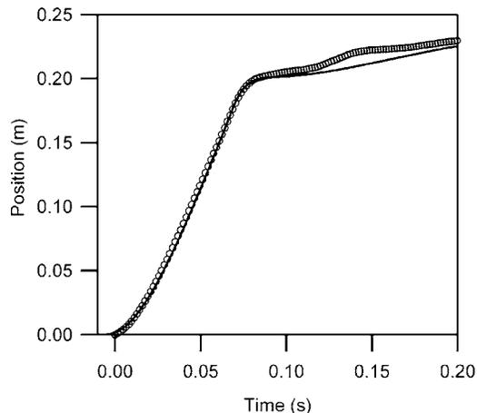
FIG. 6. Position vs time measurement and model for helium gas at 40 psig. The markers are the measured points and the line is the modeled velocity.
