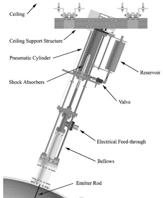
FIG. 2. Detailed view of the retracting electron emitter system.
