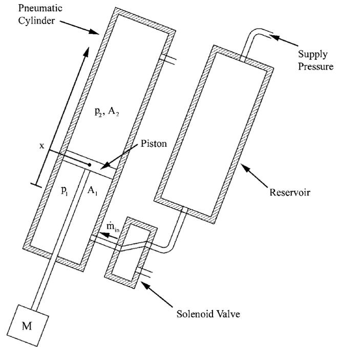
FIG. 4. Schematic of the pneumatic system.
