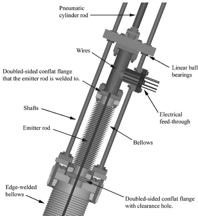
FIG. 3. Cut-away view of the bellows and emitter rod system.
