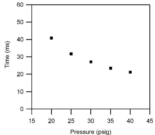
FIG. 8. The time that the emitter tip spends between the magnetic axis and the last closed flux surface vs pressure.
