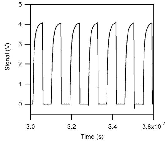
FIG. 5. Voltage on the photomicrosensor vs time. Each positive-slope crossing of 2 V represents a movement of 0.1 in.
