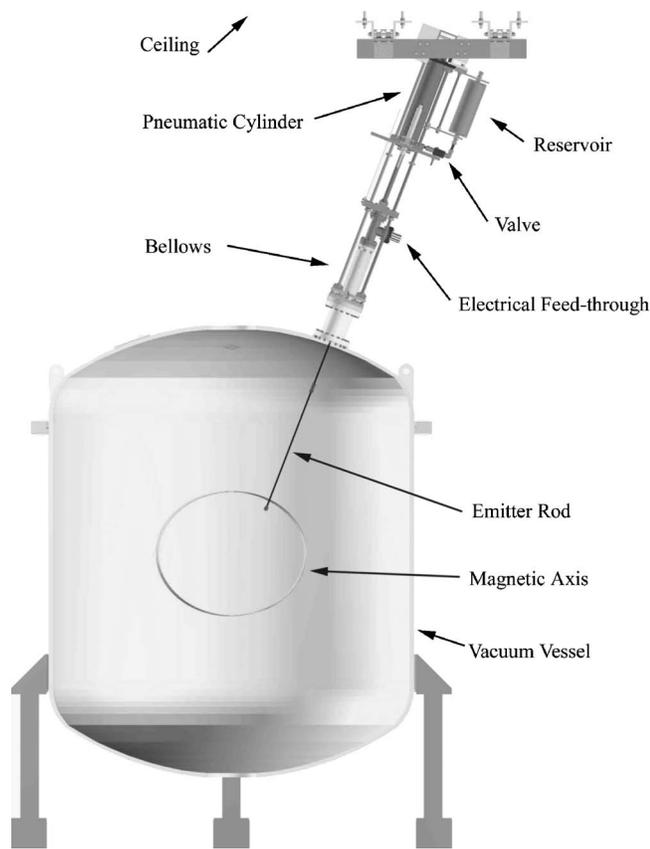
FIG. 1. Full view of the retracting electron emitter system, including a cut-away view of the vacuum tank, and a representation of the magnetic axis.
