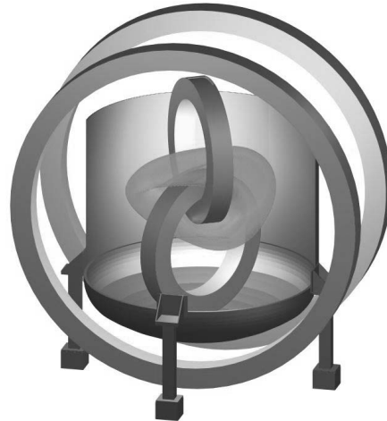
Figure 1. A cutaway CAD drawing of the Columbia Non-neutral Torus. Included are the vacuum vessel (cut in half), the two outer poloidal field coils, the two inner interlocking coils, and the rendering of the last closed magnetic flux surface.
