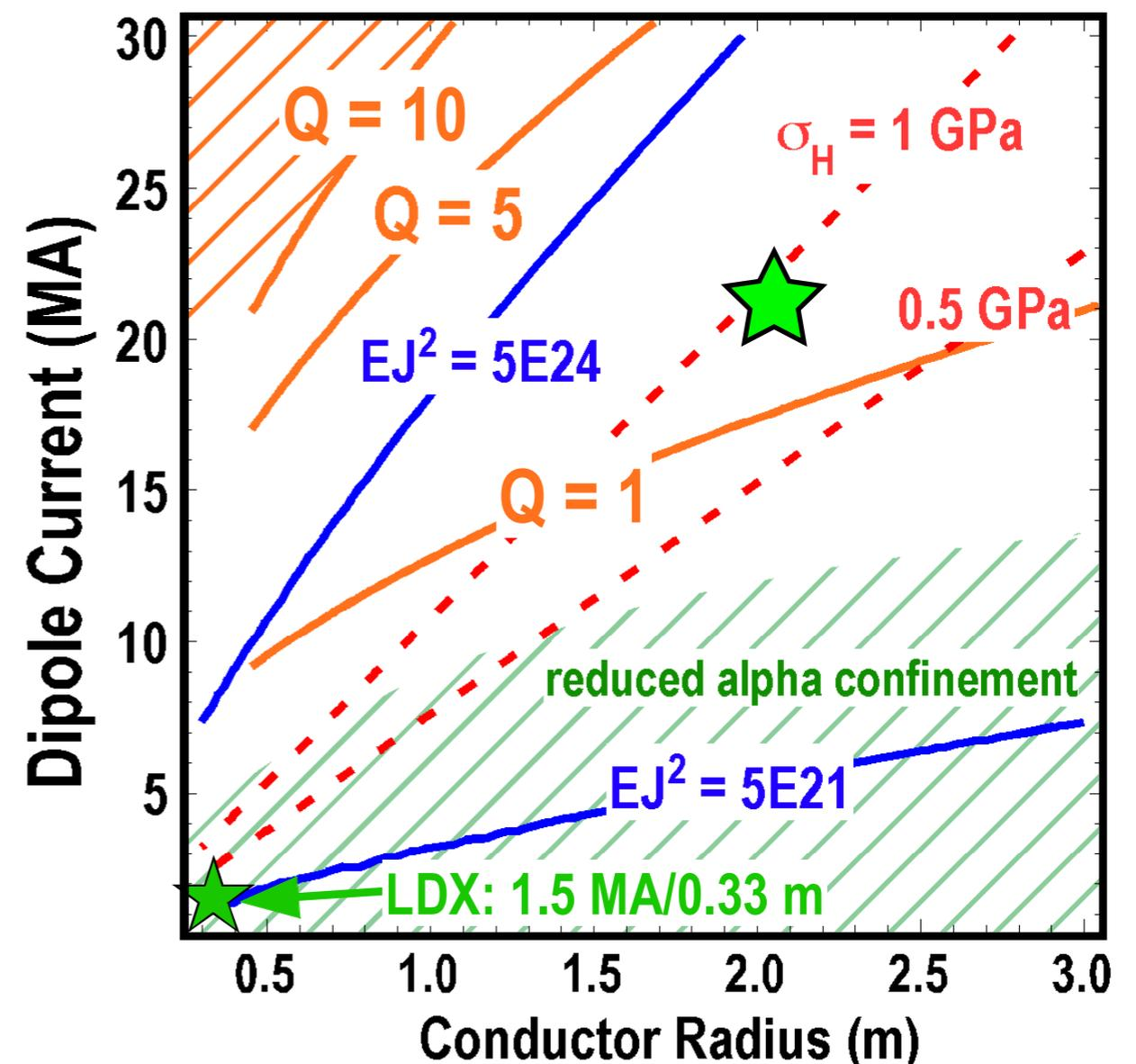
Fusion Gain - Magnet Stress - Quench Safety Parameter - Alpha Confinement
