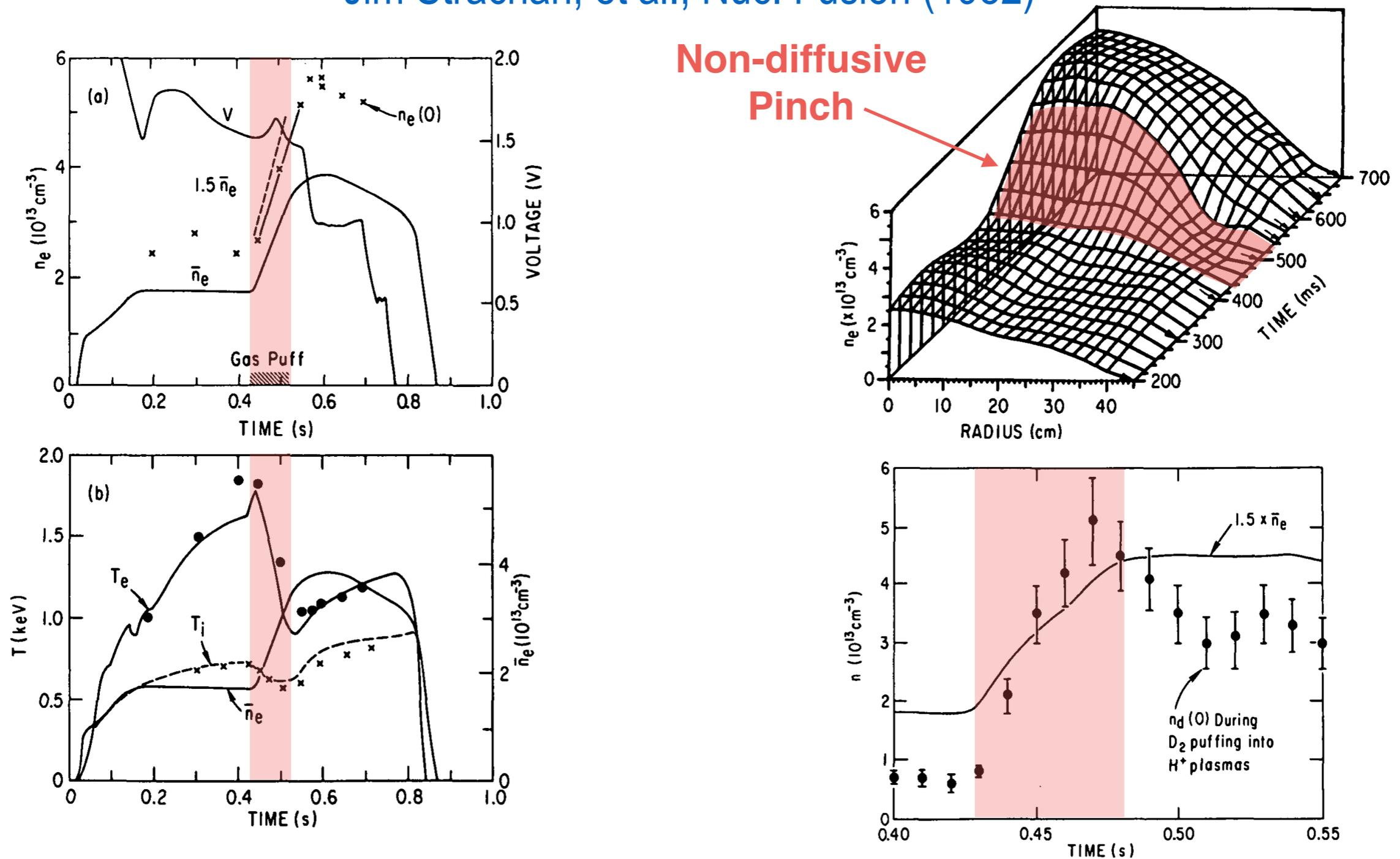
FIG.2. (a) Time evolution of the loop voltage,  $V$ , the line-average density  $\bar{n}_e$ , and the central electron density,  $n_e(0)$  during the density rise. (b) Time evolution of the central electron temperature from  $2\omega_{ce}$  (—), and from TVTS ( $\bullet$ ), with the time evolution of the central ion temperature from neutrons (—), and from charge exchange (X) during the density rise.
